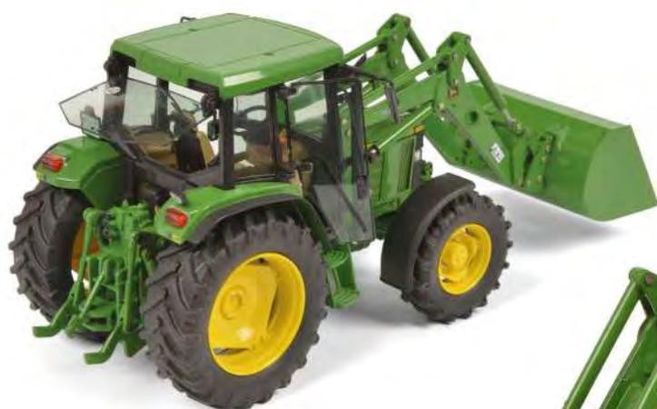
• Featuring a 100 hp engine, the John Deere 6400 was the most powerful model in the hugely popular John Deere 6000 series from the 1990s. However, the bestselling model in the series was the John Deere 6300, which had a 3920 cm<sup>3</sup> 4-cylinder diesel engine with an output of 90 hp. Built between 1992 and 1997, the 6300 had an unladen weight of 3750 kg and maximum permission gross laden weight of 7500 kg. The 1:32 edition Schuco metal model features an additional moveable front loader.
